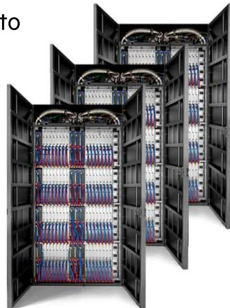
**GPU partition** with up to 448 GPUs per cabinet
